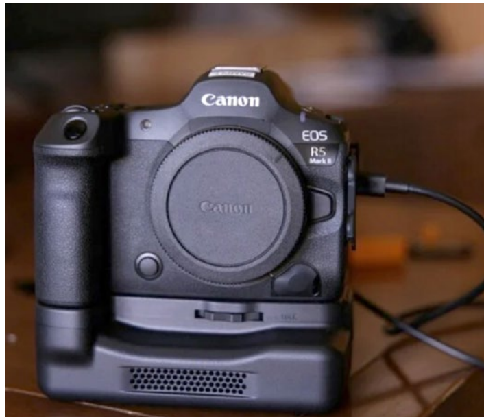
The new CF-R20-EP fan grip will keep the camera cool when sustained record times are needed.
